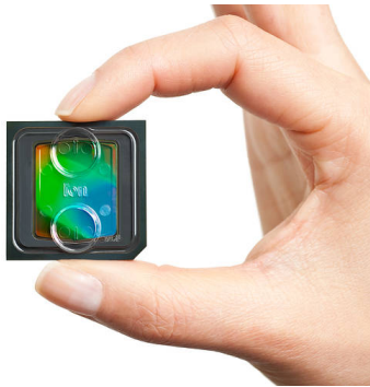
A sequencing chip from Thermo Fisher Scientific uses semiconductor technology to detect DNA associated with cancer and inherited disease. PHOTO: THERMO FISHER SCIENTIFIC
