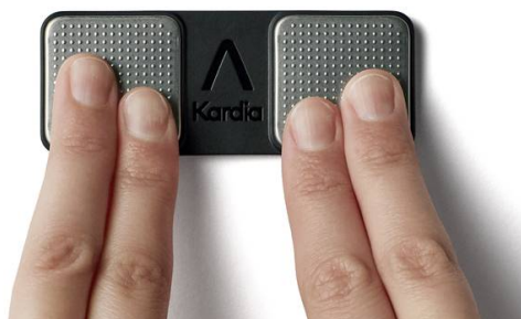
AliveCor’s Kardia traces a person’s heart rhythm on a smartphone through fingers on a sensor. PHOTO: ALIVECOR
