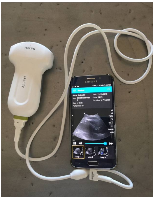
This Philips ultrasound probe connects with a smartphone. PHOTO: ERIC TOPOL
